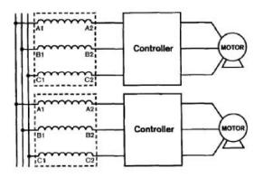
Conventional Line side reactor to VFD connections
