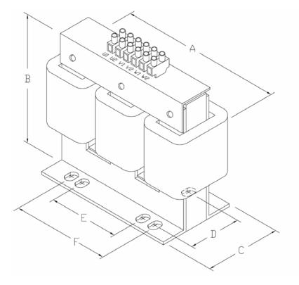
**Figure 3 Standard Mounting**
