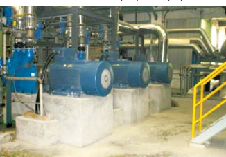
Disc refiner drivers in a pulp and paper mill
