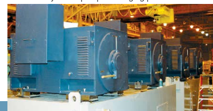
800 HP on hydraulic pumps for forging presses
